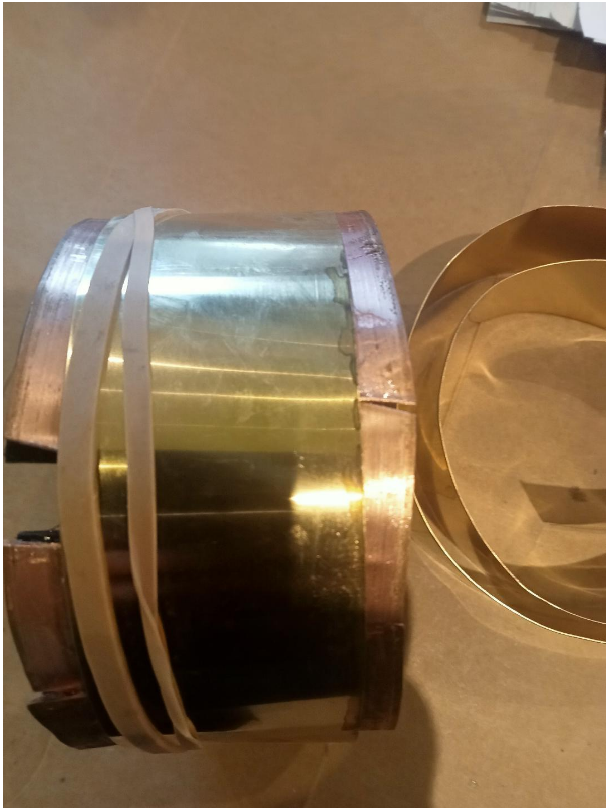
The brass has arrived! It is in a very tight coil, so I have opened it out and left it overnight stressed by an elastic band and the pegs again.
